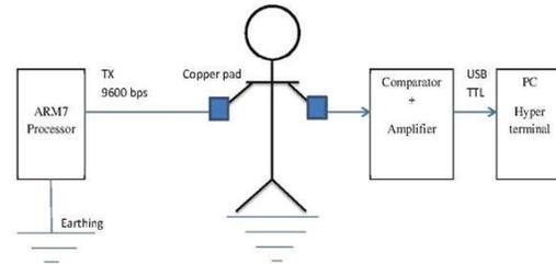
Figure 1. Experimental setup for data transfer
