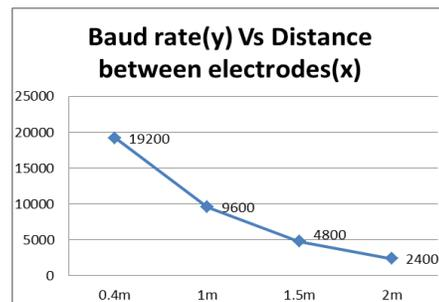
Figure 4. Graph of baud rate versus distance between electrodes
