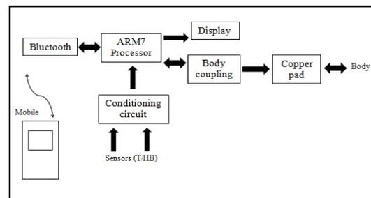
Figure 2. Hardware architecture of the proposed system
