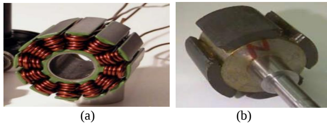
Figure 14: BLDC concentrated stator winding and PM rotor (Trapezoidal SPMSM)
