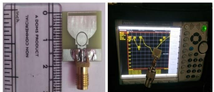
Figure 6: Photograph of Fabrication and Measuring of Proposed Antenna
