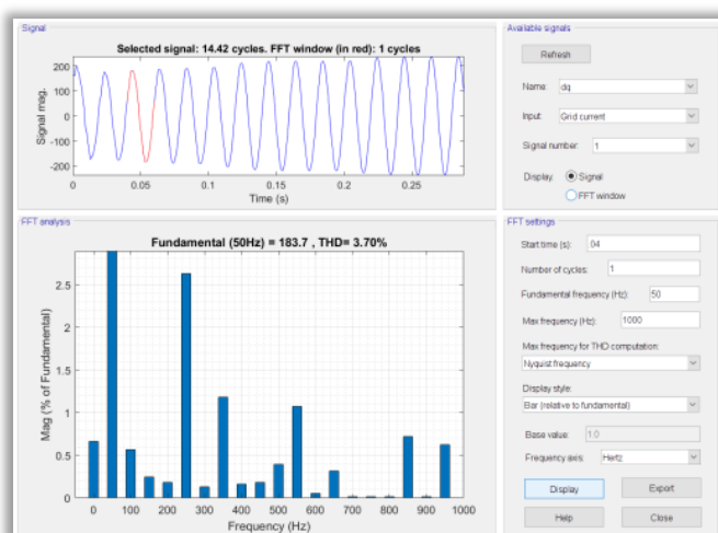
Figure 23: Grid Current THD nonlinear load and LCL filter
