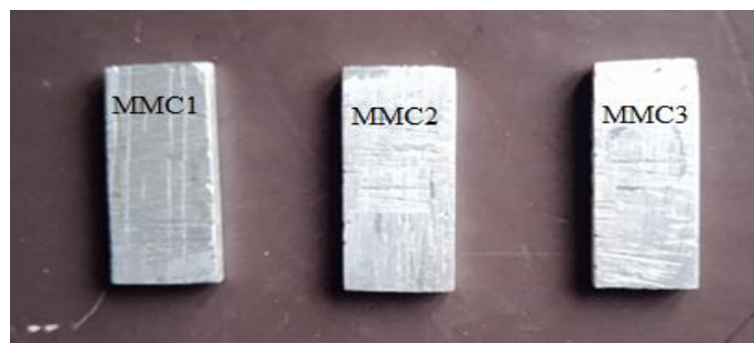
Figure 2: Fabricated Material from Stir Casting
