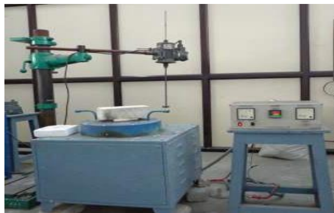
Figure 1: Experimental setup for reinforcement using stir casting
