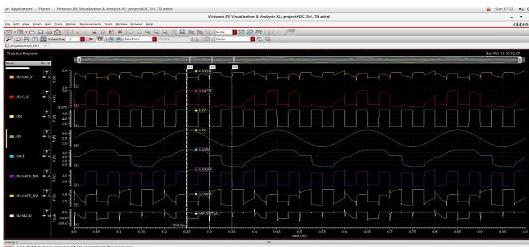
Figure 9: Signals and Transient Response of S&H in cadence
