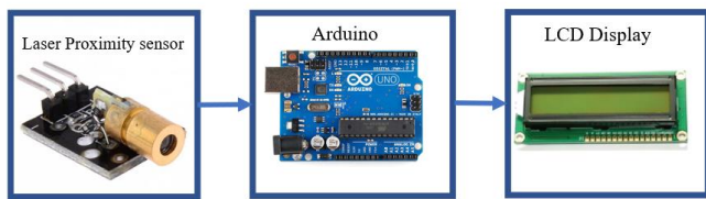
Fig. 6a: Prototype of laser proximity sensor and LCD
