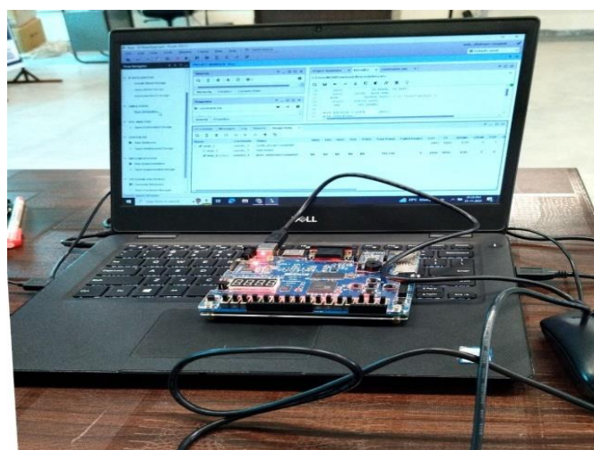
Figure 11. AES/SHA3-512 FPGA Output Implementation Display and hardware Setup
