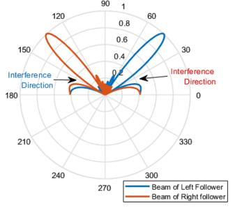
**Figure 8.** The Beamforming Response Main Loops directed to Leader Angle (45<sup>0</sup>, 135<sup>0</sup>) for Left and Right Follower respectively, the Direction of Interferences are Ignored with Null (Zero Power)
