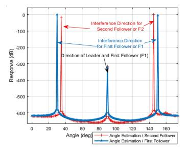
Figure 12. The Estimation Response for the Two Robots
