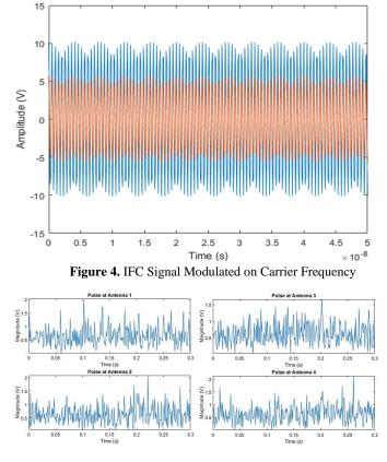
Figure 5. The Received Signal at each Antenna in the MIMO Array of Four Antenna
