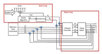
Figure 3. Flying Robot Control System
