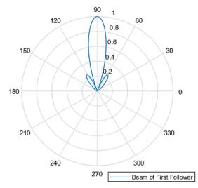
Figure 13. The Beamforming Response of the First Follower
