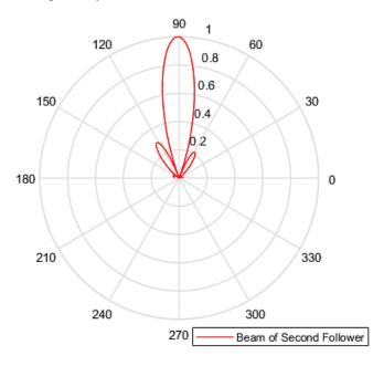
Figure 14. The Beamforming Response of the Second Follower
