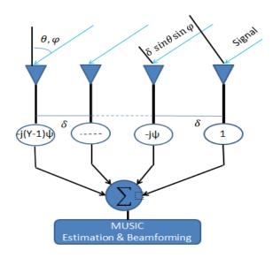
Figure 2. Array of Antenna configuration and phase estimation
