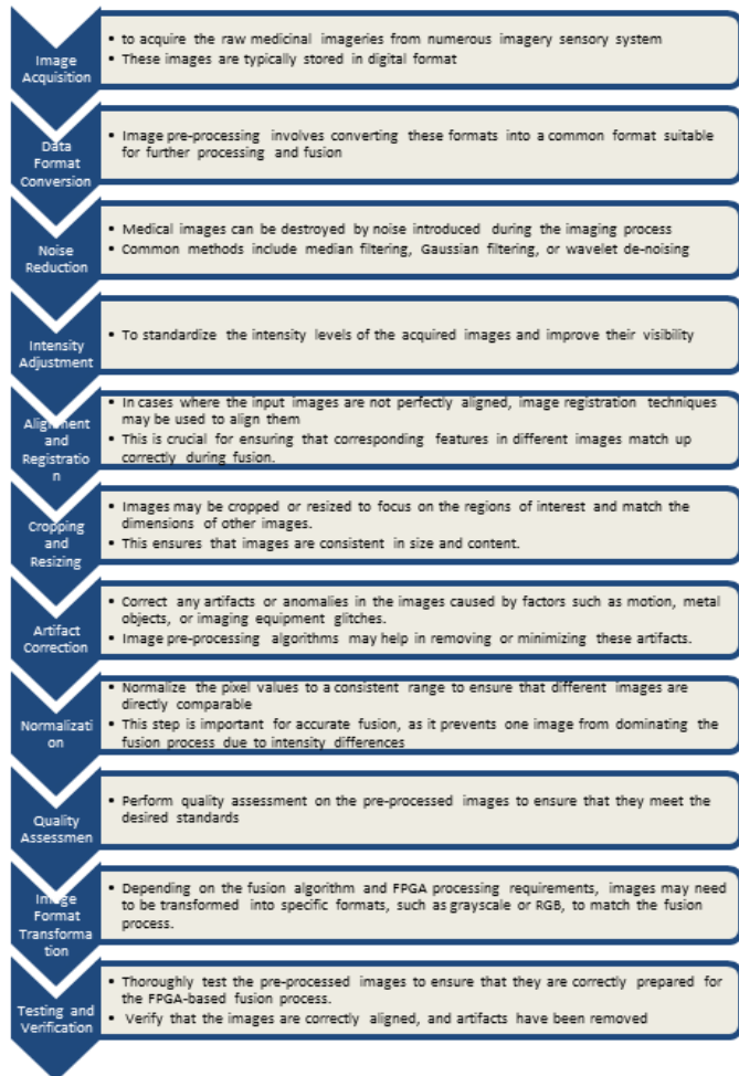
Figure 2. Pre-processing steps for image fusion
