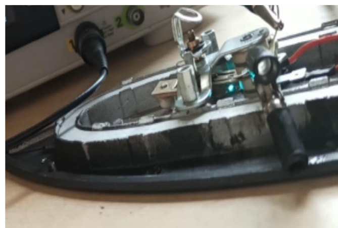
Figure 23. Arcing across the switch with capacitor
