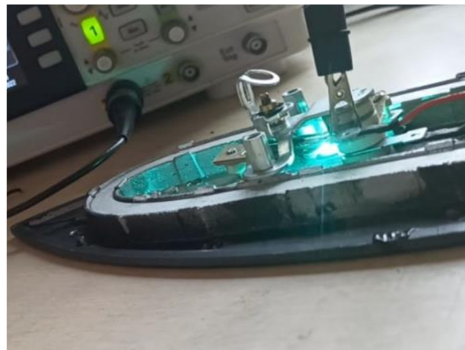
Figure 22. Arcing across the switch without capacitor
