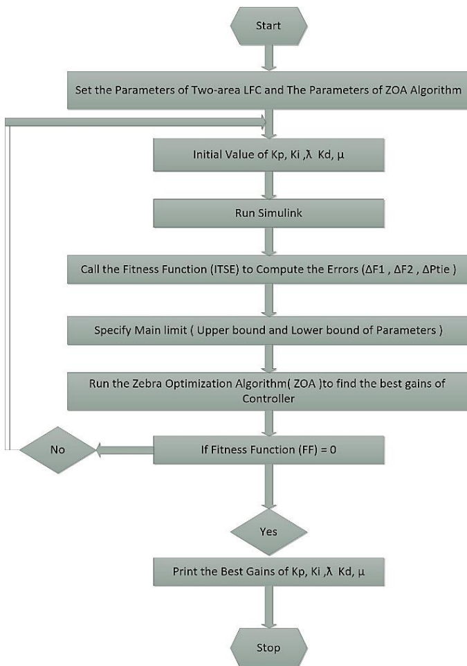
Figure 6. Fractional Order Proportional Integral Derivative with Zebra Optimization Algorithm Flowchart
