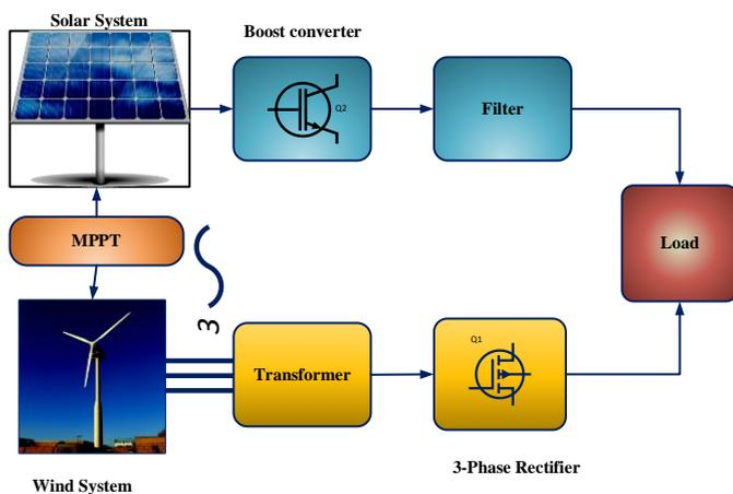
**Figure 1.** Block diagram representation of hybrid energy system
