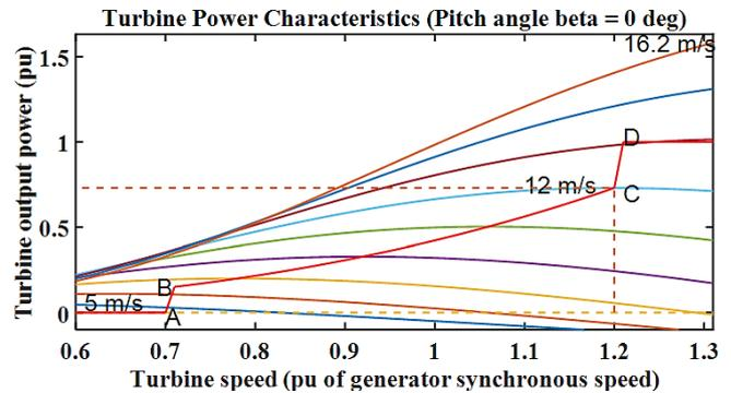
**Figure 6.** Representation of wind turbine characteristics
