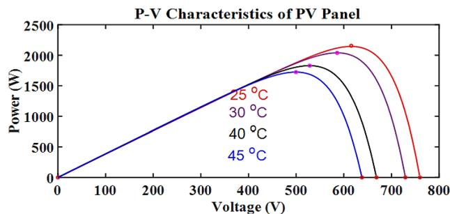
**Figure 5.** representation of P-V characteristics of solar panel
