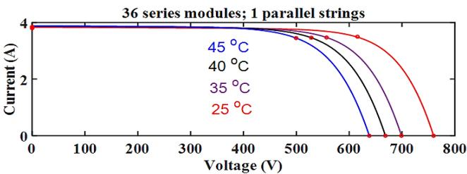
**Figure 4.** Representation of I-V characteristics of solar panel
