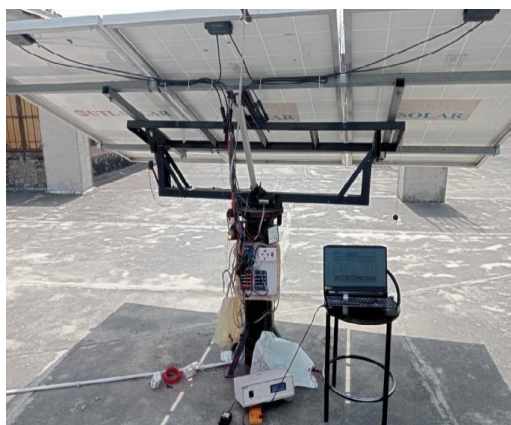
Figure 10: Hardware Set up of Data Acquisition (DAQ) or String Monitoring System with a 200- watt load
