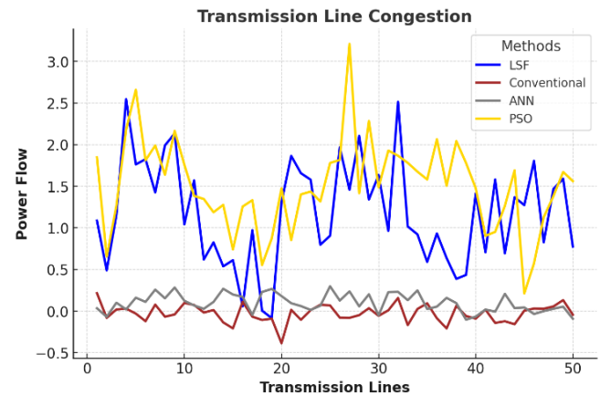
Figure 2. Transmission line Vs Power flow for Conventional, LSF, PSO and ANN methodologies representing congestion scenario
