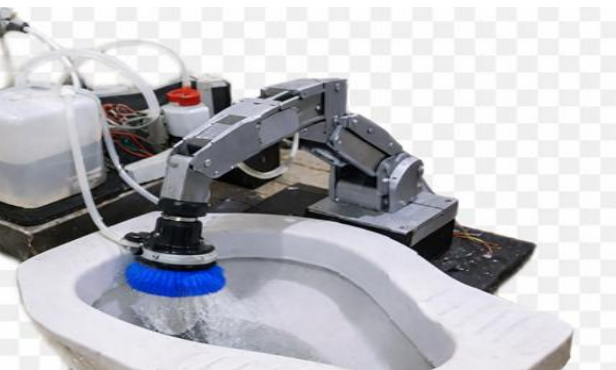
Figure 11. AI-IoT Robotic cleaning the Indian style toilet pot
