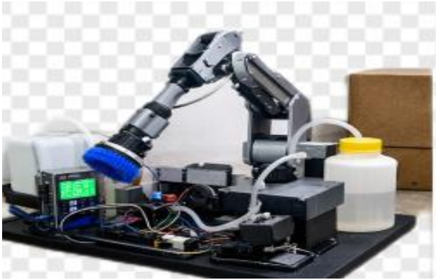
Figure 9. Complete cleaning system
