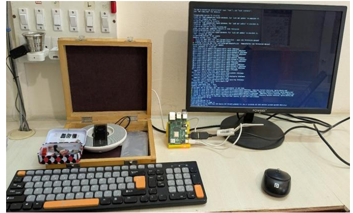
Figure 4. Hardware of MPC based MIMO system
