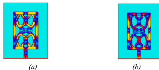
Figure 6. Surface current distribution at frequencies (a) 11.347 GHz and (b) 12.809 GHz on the surface of the suggested antenna
